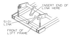
2. Remove front and rear deck hanger pins, as illustrated below.
